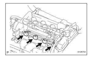
(3) Using a 16 mm plug wrench, remove the 4 spark plugs.
