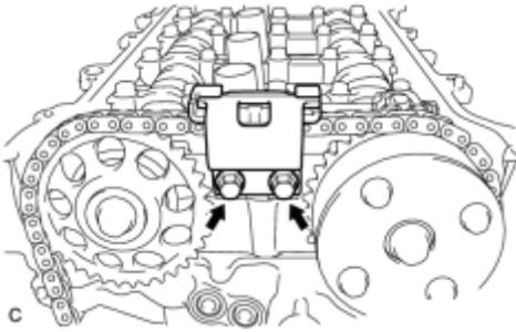
14. INSTALL CHAIN TENSIONER SLIPPER
