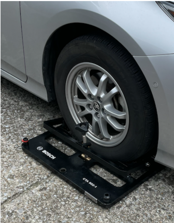
The first step setting up the Bosch CTA 410 alignment rig
